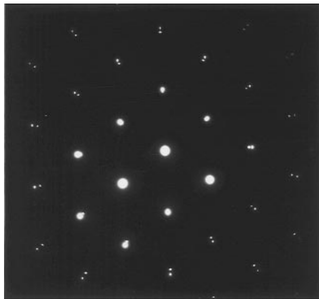
Figure 4. Typical selected area electron diffraction pattern of \text{Ge}_{0.97}\text{C}_{0.03}/\text{Si} showing highly ordered \text{Ge}_{1-x}\text{C}_x layer with diamond cubic structure.
